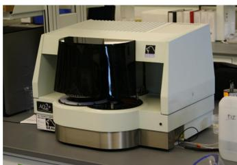
Figure 2 - SEAL AQ2+ Auto Analyzer
