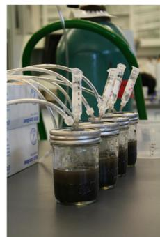
Figure 3 - Helium flushing during DEA
